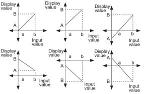
Display scale function is able to change display value for max./min. measured input by setting high limit scale [H-5E] and low limit scale [L-5E] in program mode.
