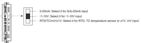
This unit is multi input product. Select the proper input with the input type selection switch and select this input type in  $l n^{-P}$  in program mode. The setting of input type selection switch and the input type  $l n^{-P}$  parameter should be same and it can display the proper measurement value. Factory default is 0-20mA.
